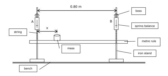
3. Position the 200-g mass provided at x = 0.30 m and take note of the reading of both spring balances.
